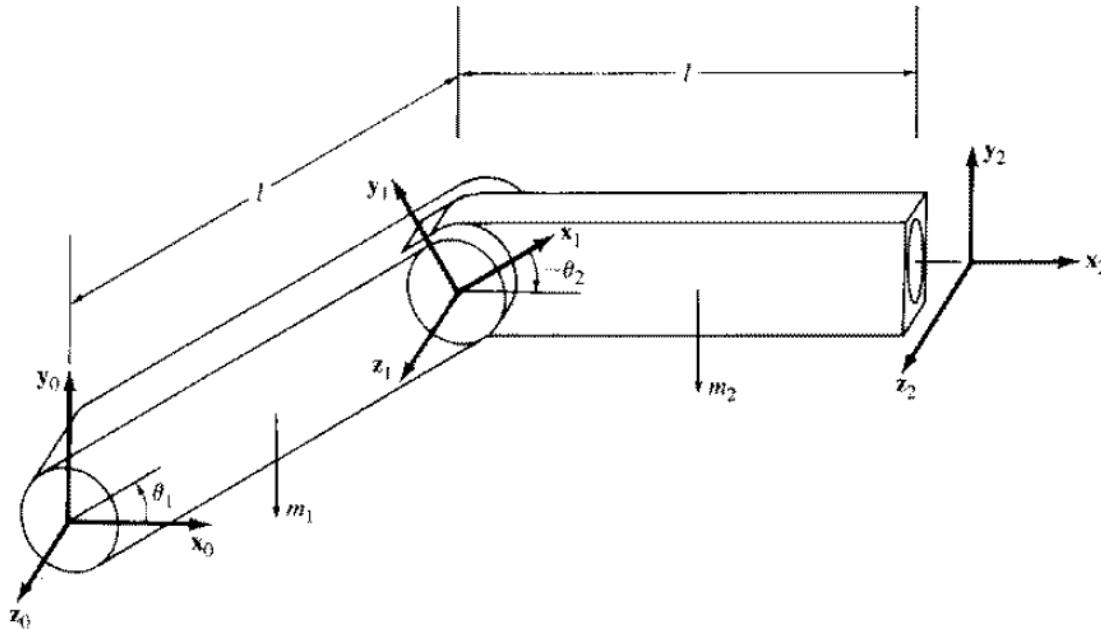
$${}^0\mathbf{A}_1 = \begin{bmatrix} C_1 & -S_1 & 0 & lC_1 \\ S_1 & C_1 & 0 & lS_1 \\ 0 & 0 & 1 & 0 \\ 0 & 0 & 0 & 1 \end{bmatrix} \quad {}^1\mathbf{A}_2 = \begin{bmatrix} C_2 & -S_2 & 0 & lC_2 \\ S_2 & C_2 & 0 & lS_2 \\ 0 & 0 & 1 & 0 \\ 0 & 0 & 0 & 1 \end{bmatrix}$$
