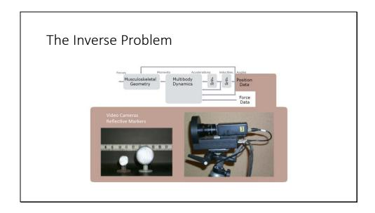
If we know the positions of three points on a rigid body in three-dimensional space, we can completely determine that rigid body's position and orientation. Our marker set is designed to give us the locations of at least three markers on each rigid body segment so that the position and orientation of each body segment of interest can be completely determined. To this end, motion capture systems (Vicon, Motion Analysis) are used to track the position of the markers attached on the body.
