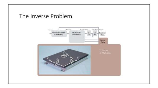
External load data (i.e., ground reaction forces, moments, and center of pressure location). Note that it is necessary to measure and apply or model all external forces acting on a subject during the motion to calculate accurate joint torques and forces.
