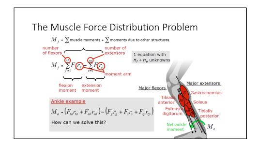
Many unknowns in one equation. Solution to this unconstraint problem can be achieved, by introducing additional equations, constraints and an objective function that we want to minimize.
