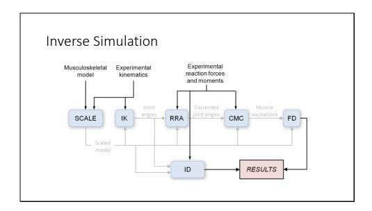
OpenSim enables researchers to solve the Inverse Dynamics problem, using experimental measured subject motion and forces to generate the kinematics and kinetics of a musculoskeletal model (see figure below). In inverse dynamics, experimentally measured marker trajectories and force data are use to estimate a model's kinematics and kinetics.
