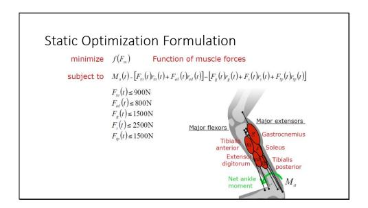
Minimize some objective function, so that the muscle forces will produce the desired torque around a joint, while accounting for the force capability of each muscle.
