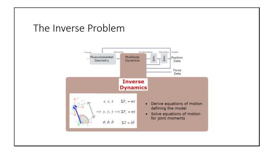
Classical mechanics mathematically expresses the mass-dependent relationship between force and acceleration,  $\mathbf{F} = m\mathbf{a}$ , with equations of motion. The Inverse Dynamics (ID) Tool solves these equations, in the inverse dynamics sense, to yield the net forces and torques at each joint which produce the movement.
