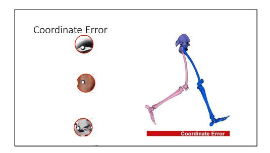
A *coordinate error* is the difference between an experimental coordinate value and the coordinate value computed by IK.
