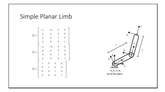
This limb is anchored to ground, where ground is the base frame, or frame 0. The first DOF (i.e., q1) rotates the first link in a positive (as per the right-hand-rule) direction. The second DOF (i.e., q2) rotates the second link with respect to the first link. This is an important convention in kinematic analysis in robotics: the generalized rotational coordinates qi are relative to the prior body.
