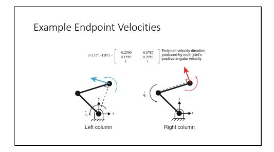
Illustration of the Jacobian for a 2 DOF planar limb. For the posture shown, the columns of the 2  $\times$  2 Jacobian show the expected *instantaneous* endpoint linear and angular velocity for isolated angular velocities of 1 rad/s at each of the joints. If both joints are actuated, then their contribution to instantaneous endpoint velocity simply add. The limb parameters are, as per the convention in Fig. 2.3, li = 25.4cm, l2 = 30.5cm,  $q1 = 135^{\circ}$ , and  $q2 = -120^{\circ}$ .
