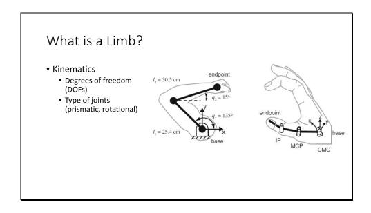
Human arm model modeled as planar 2DOF serial manipulator.
