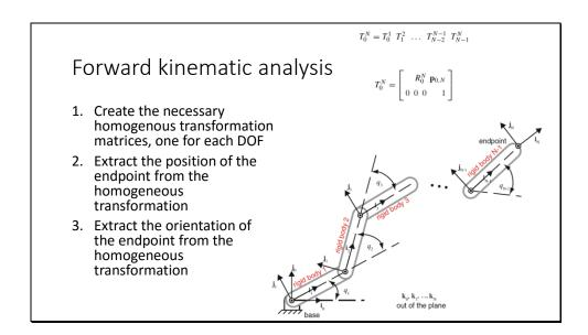
The forward kinematics of a limb determine the location and orientation of its endpoint with respect to its base, given the relative configurations of each pair of adjacent links of the limb.
