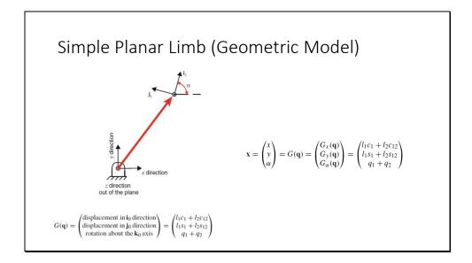
Therefore, in this case the forward kinematic model (also called the geometric model),  $G(\mathbf{q})$ . It defines the position and orientation of the end effector.
