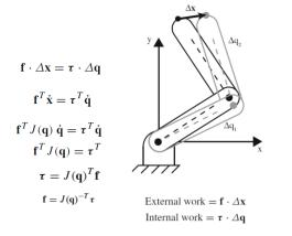
Defining the static force production capabilities of limbs begins by deriving the equation that determines the production of wrenches at the endpoint as a function of joint torques. Recall that the mechanical output of the last link of a limb can be both forces and torques (i.e., the endpoint wrench). This equation is derived using the principle of virtual work, a corollary of the law of conservation of energy.
