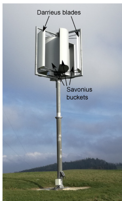
Figure 7. H-Darrieus turbine with hybrid rotor configuration [78].
