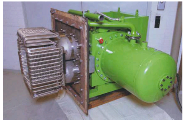
Fig. 6. Picture of 35-kW SE [48].
