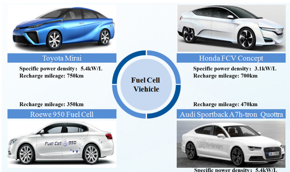
Fig. 17. Representative FCVs: Toyota Mirai, Honda FCV Concept, Roewe 950, and Audi A7 (The specific power density of Roewe 950 and Audi A7h are not given in public resources) (Nonobe, 2017).
