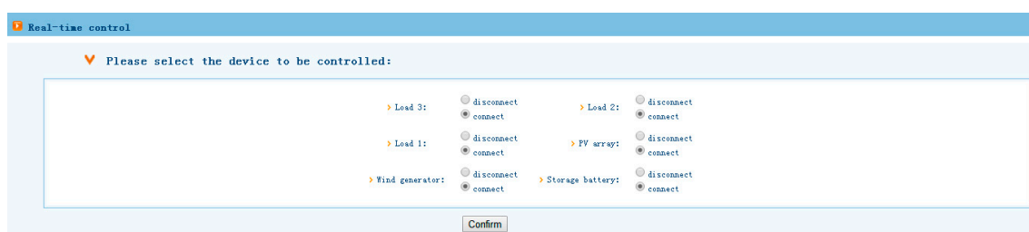
Figure 12. Real-time control user interface in the WEB monitoring system.
