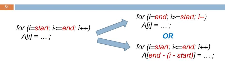
Loop reversal is a transformation that reverses the order of the iterations of a given loop
