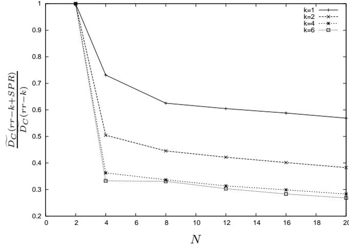
Fig. 6. Ratio of the Overall confirmation delay for the rr-k+SPR protocol and the rr-k protocol  $\frac{\overline{D}_C(rr-k+spr)}{\overline{D}_C(rr-k)}$  vs. number of wireless stations  $N$  for 50% low priority load and complex error model
