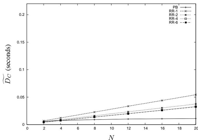
Fig. 5. Overall confirmation delays  $\widetilde{D}_C$  for rr- $k$ -protocols and the PROFIBUS protocol vs. number of WT's  $N$  for 10% background load and the independent error model.
