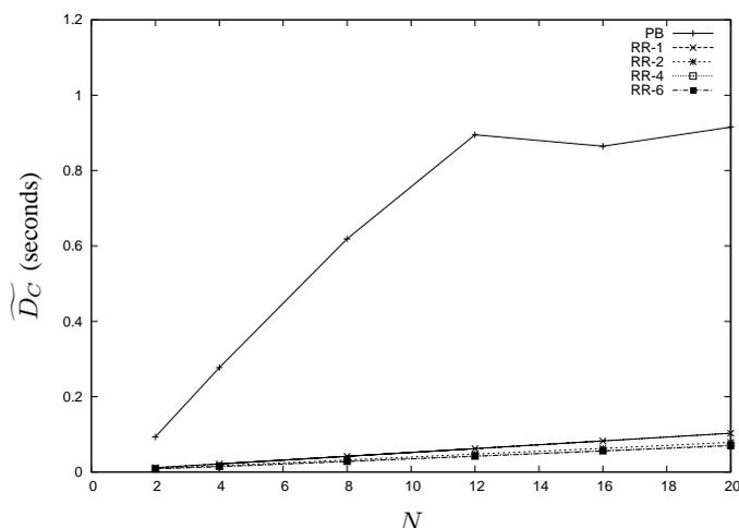
Fig. 4. Overall confirmation delays  $\widetilde{D}_C$  for rr- $k$ -protocols and the PROFIBUS protocol vs. number of WT's  $N$  for 10% background load and the Gilbert-Elliot error model.
