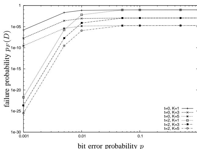
Fig. 7. Failure Probabilities vs. bit error probability  $p$  during bad state for the experiment ‘Efficiency of Redundancy Approaches’,  $t \in \{0, 2\}$
