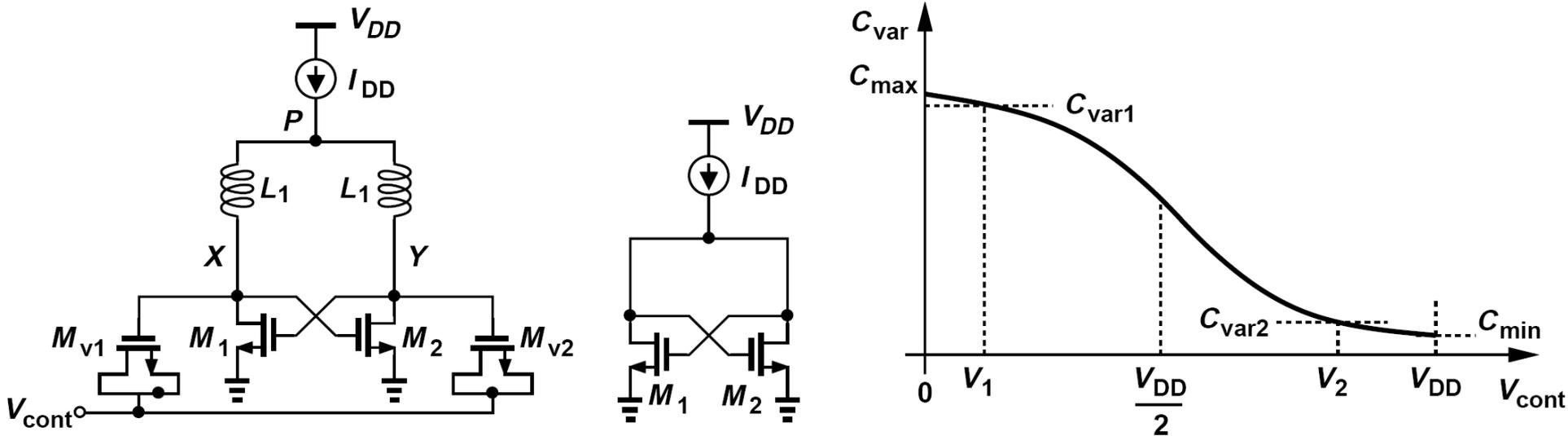
The CM level is simply given by the gate-source voltage of a diode-connected transistor carrying a current of  $I_{DD}/2$ .
