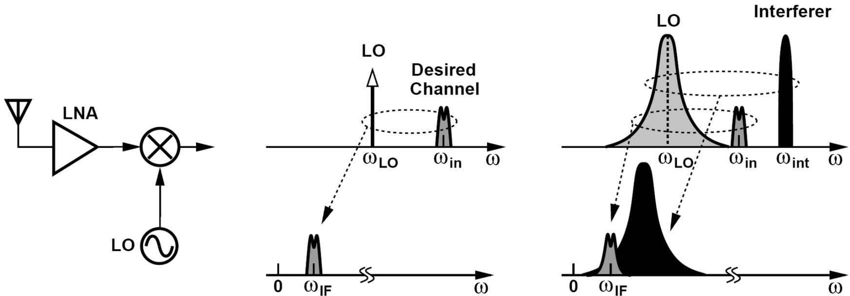
➤ Referring to the ideal case depicted above (middle), we observe that the desired channel is convolved with the impulse at  $\omega_{LO}$ , yielding an IF signal at  $\omega_{IF} = \omega_{in} - \omega_{LO}$ .
