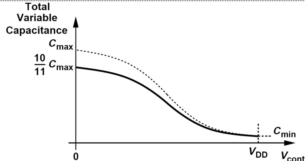
➤ The principal drawback of the above circuit stems from the parasitics of the coupling capacitors.
