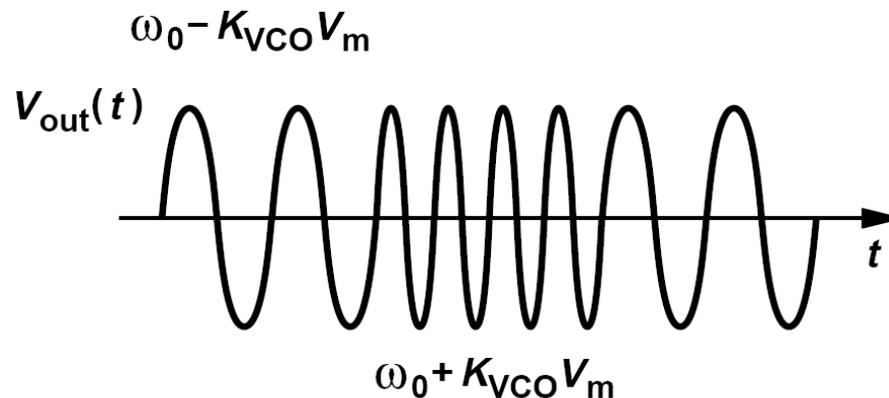
As an example, suppose  $V_{cont} = V_m \sin \omega_m t$ , i.e., the frequency of the oscillator is modulated periodically. Intuitively, we expect the output waveform frequency periodically swings between  $\omega_0 + K_{VCO} V_m$  and  $\omega_0 - K_{VCO} V_m$ , i.e., has a “peak deviation” of  $\pm K_{VCO} V_m$ . However, the student’s expression yields
