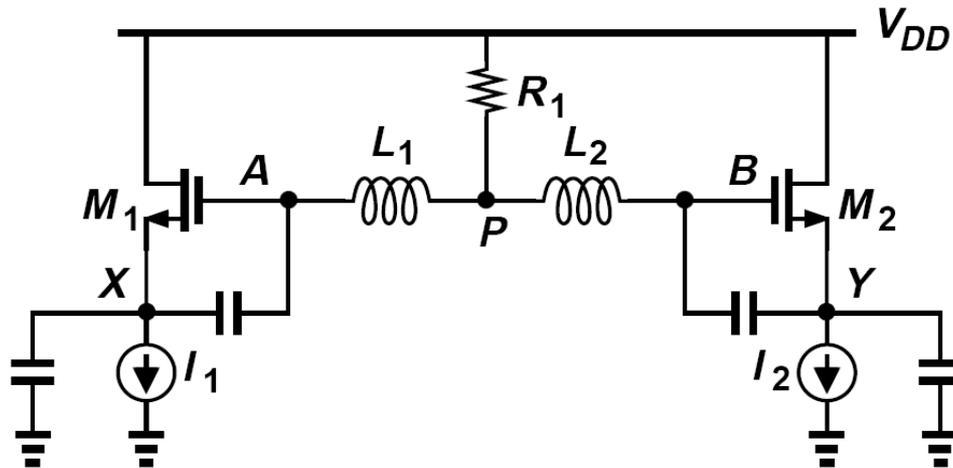
➤ If chosen properly, the resistor  $R_1$  prohibits common-mode oscillation.
