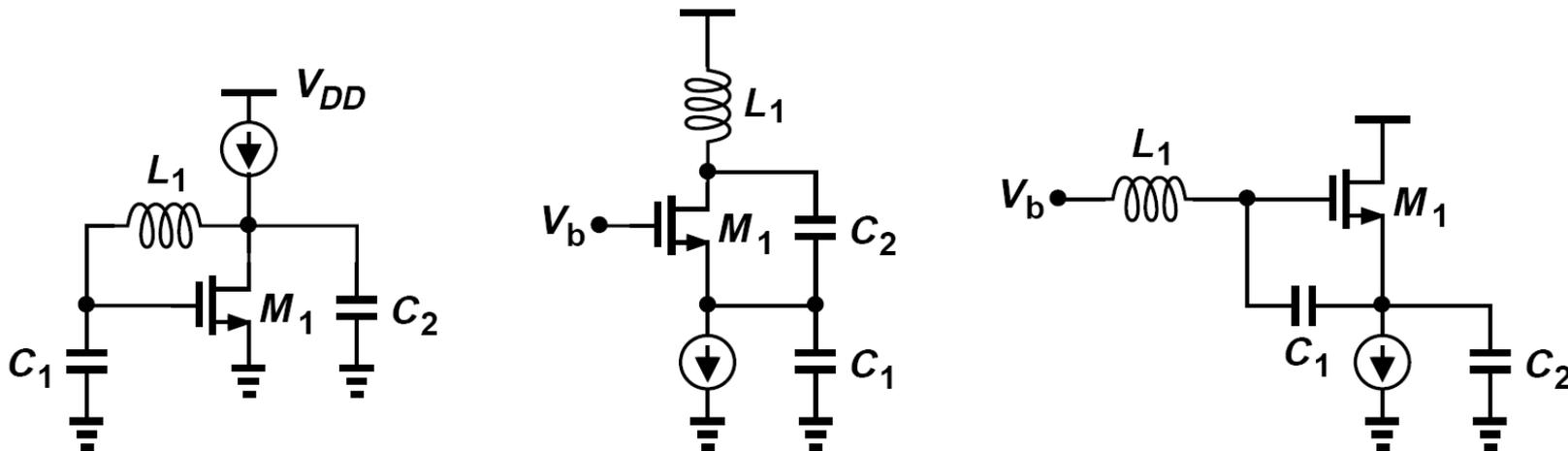
If  $C_1 = C_2$ , the transistor must provide sufficient transconductance to satisfy
