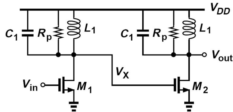
This result is to be expected: the cascade of frequency-selective stages makes the phase transition sharper than that of one stage.
