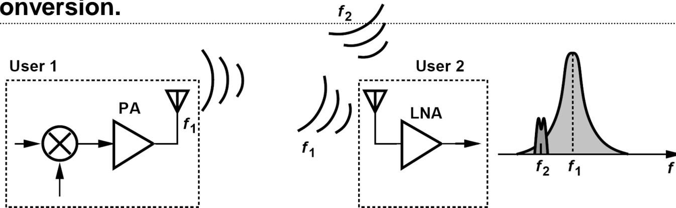
A student reasons that, if the interferer at  $f_1$  above is so large that its phase noise corrupts the reception by user #2, then it also heavily compresses the receiver of user #2. Is this true?
