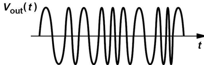
The intersection of each horizontal line with the phase plot signifies the zero crossings of  $V_{out}(t)$ . Thus,  $V_{out}(t)$  appears as shown above. The key point here is that the VCO frequency is not modulated periodically.
