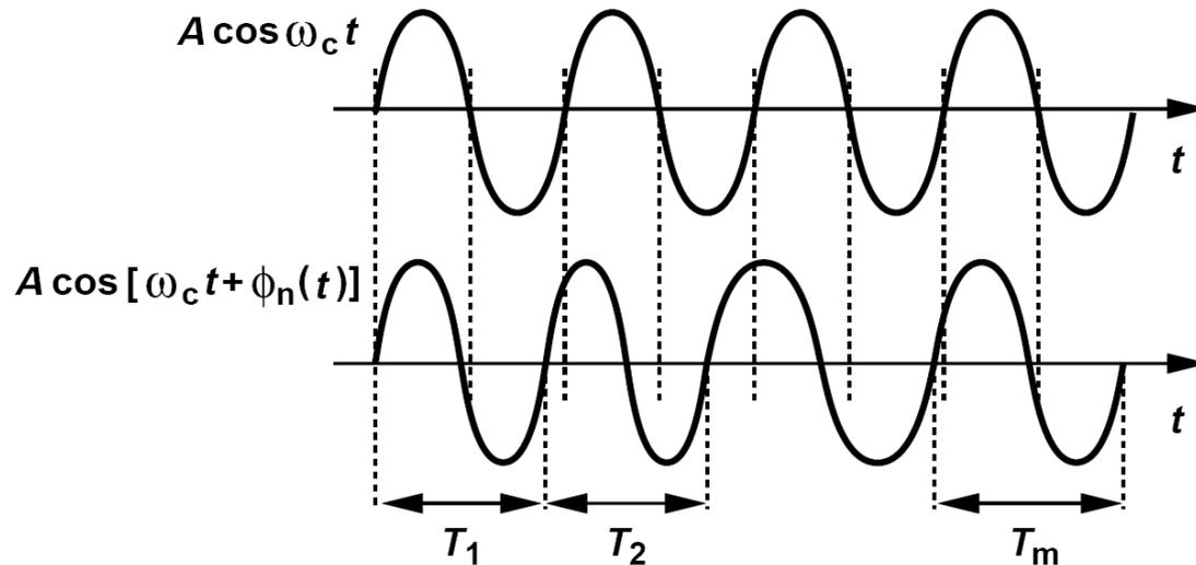
➤ The noise of the oscillator devices randomly perturbs the zero crossings. To model this perturbation, we write  $x(t) = A \cos[\omega_c t + \phi_n(t)]$ , The term  $\phi_n(t)$  is called the “phase noise.”
