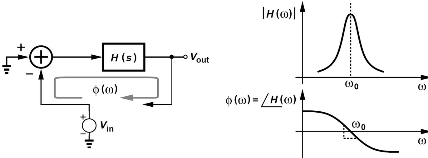
➤ Another definition of the Q that is especially well-suited to oscillators is shown above, where the circuit is viewed as a feedback system and the phase of the open-loop transfer function, is examined at the resonance frequency.
