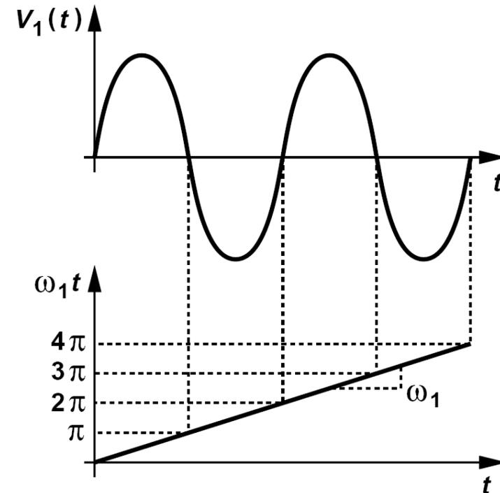
➤ A VCO is simply a frequency modulator. For example, the narrow-band FM approximation holds here as well.
