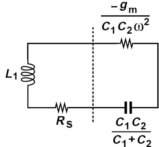
Express the oscillation condition in terms of inductor's parallel equivalent resistance,  $R_p$ , rather than  $R_S$ .
