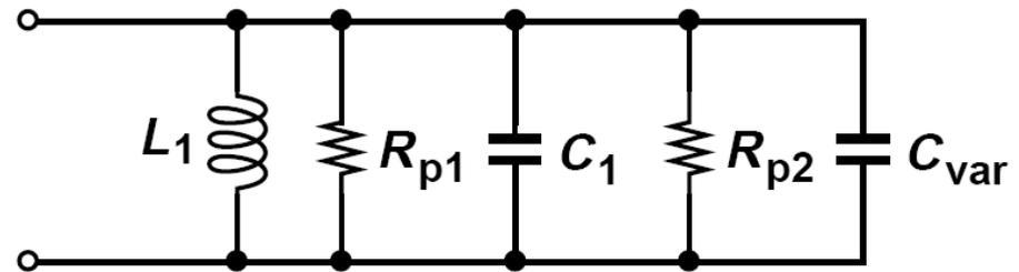
Transforming the series combination of  $C_{var}$  and  $R_{var}$  to a parallel combination
