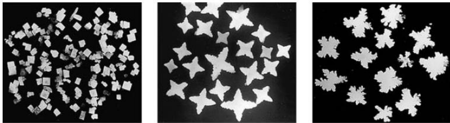
Figure 6.41. Habit changes in sodium chloride crystals caused by traces of impurity: (a) pure solution, (b) 0.1% Fe(CN) 6 4- , (c) 1% Fe(CN) 6 4- . (Cooke, 1966)
