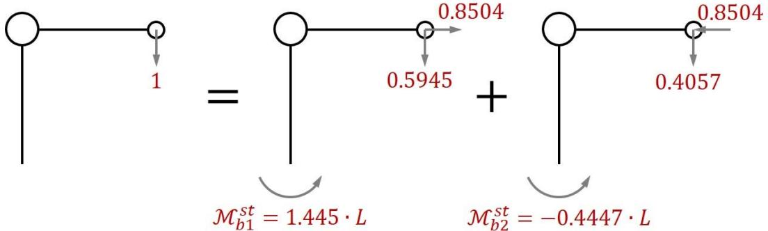
It follows that the induced static moment at the base of the column (for each mode separately):
