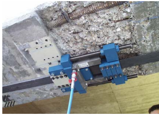
Fig. 2.9 (a) Schematic illustration and (b) photograph of FRP anchorages.
