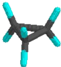
Cyclopropane Avg Bond Angle = 60^\circ Strain Energy = 114.2 kJ/mol
