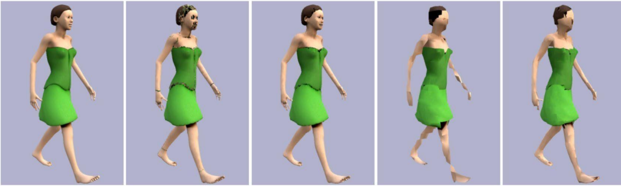
Figure 1: From left: 160,000-triangle textured model; simplification by vertex clustering to 30,000 triangles in 40ms, causing artefacts at UV seams; artefacts eliminated by our algorithm in an additional 7ms; heavy simplification causing blockiness and dropouts in 13ms; improved by our extended algorithm in 3ms.
