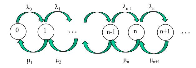
It can be shown that when the system is in steady state, the total flow into any state n is equal to the total flow out of that state i.e.
