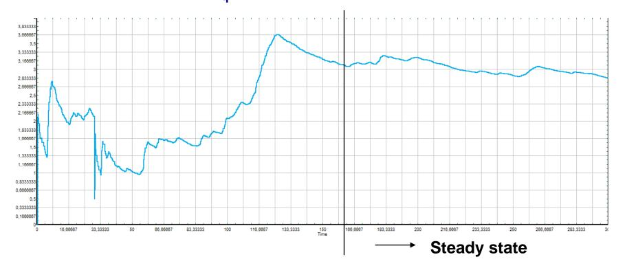
Steady state: the state where the probability of the number of customers in the system (or in the queue) is independent of time
