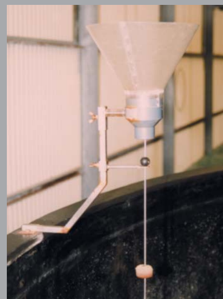
Fig.63.02 Demand feeders are used with bigger size pellets (photo STM Aquatrade)
