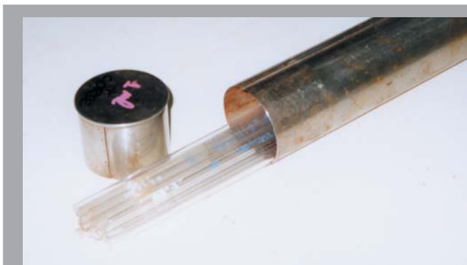
Fig. 24.05 Pipette container used with oven sterilization (photo STM Aquatrade)
