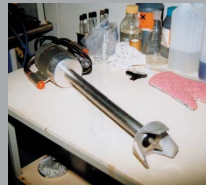
Fig. 30.04 An industrial blender for yeast or Culture Selco® suspension (photo STM Aquatrade)
