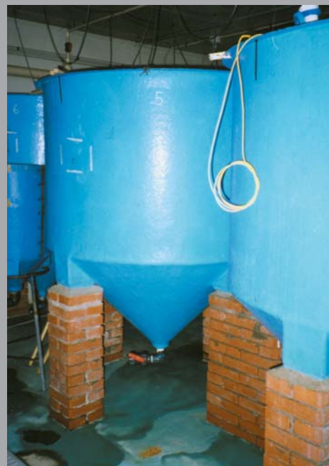
Fig. 30.00 The classic cylindroconical rotifers tank (photo STM Aquatrade)
