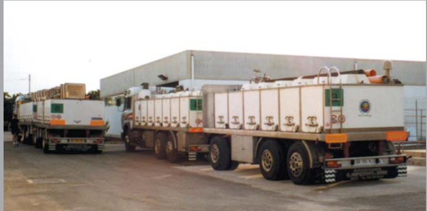
Fig.69.01 Fry transportation trucks (photo STM Aquatrade)
