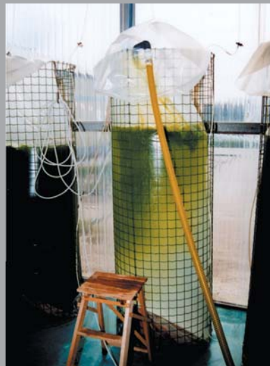
Fig. 25.07-08 PE bags inoculation with the help of a self-priming pump (photo STM Aquatrade)
