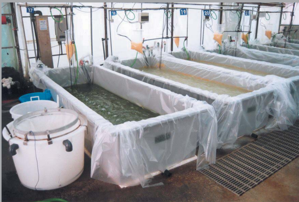
Fig. 30.07 CS distribution by gravity to the tanks at Ittica Ugento (photo STM Aquatrade)
