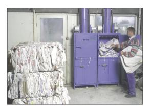
Compacting Compacting is a standard industry technique which can be used to reduce the volume of waste on a fish farm. This is especially useful in the volume reduction of cardboard and polystyrene fish boxes
