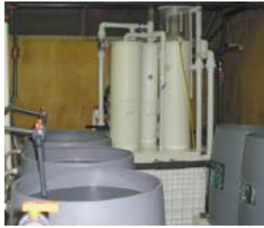
Seahorses Seahorse cultivation requires stringent water quality. Recirculation technology ensures a stable environment for the seahorses with optimum conditions resulting in improved growth and survival rates.
