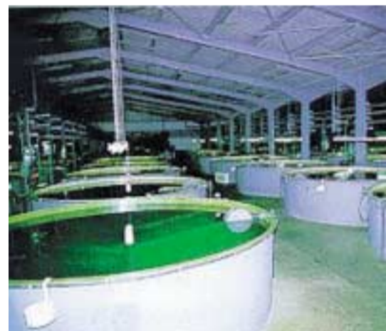
1 Culture Tank Most culture tanks in recirculation systems are made of circular fibreglass. These tanks are designed to minimize the water residence time in the tank and maximize the feed and waste removal. Some water exits the bottom of the tank, taking with it the bulk of the waste particles in the form of sludge. The bulk of the water however leaves to be treated in the system below.
