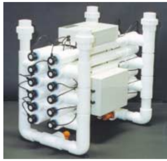
7 UV Sterilisation Disinfection of recirculated water is achieved through ultraviolet (UV) irradiation. When water is passed through the UV steriliser above, microorganisms in the water come into contact with UV radiation emitted into the channels. The UV radiation penetrates the cell membranes, either destroying or debilitating any micro-organisms present.
