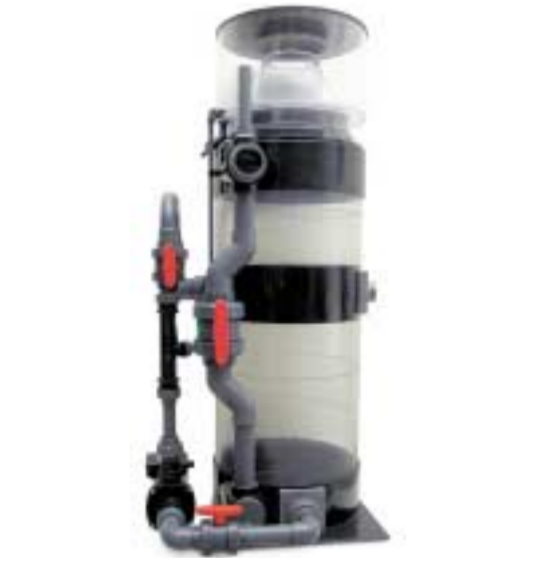
6 Protein Skimmer Proteins are extracted from the water column by vigorously mixing the water with injected air or liquid oxygen. The foam produced from this process then floats on the surface of the water and can be "skimmed". This process also aerates the water at the same time. Additional use of ozone cracks up any remaining organic material that could adversely influence the development of fish. Protein skimmers are most effective in saltwater. Freshwater systems utilise a bag filter/reactor system.
