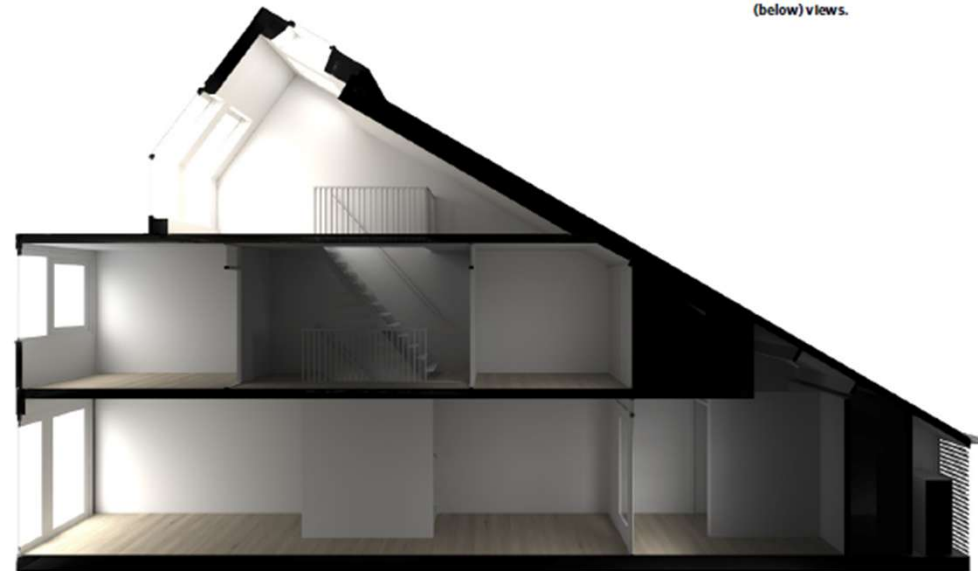
Section through one house showing the distribution of luminance levels under overcast sky conditions in photo-realistic (above) and false colour (below) views.
