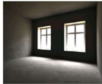
Traditional single-glazed window Daylight Factor 1,92%
