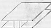
Floor/roof made from concealed squared sections plus planking, boarding or wood-based panels
