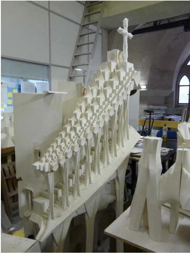
Rapid prototypes and mould of material for the construction in real scale, Sagrada Familia, 2008.
